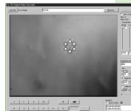
Fig. 1: Graphical user interface written in Visual C++ for a confocal microscope coupled to a CCD camera. The program allows the automated tracking of the image of colloidal beads selected by the user.
